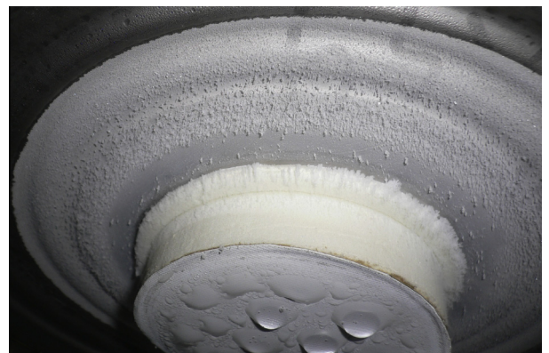
Fig. 4. Photo of specimen glued to the copper disk tightly when the supporter is just taken off.
